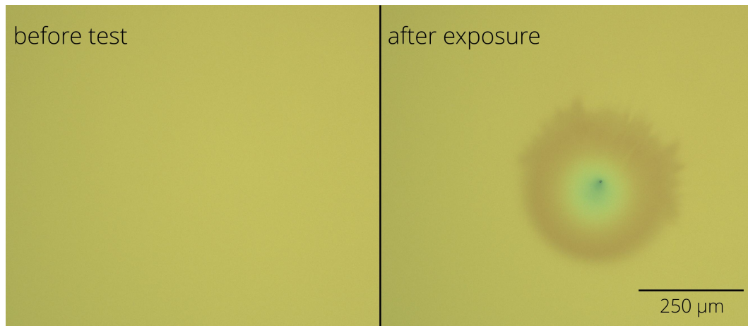
Figure 4. Typical damage morphology: fluence 158 \text{ J/cm}^2 , damage after 1 pulse(s).
