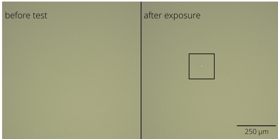
Figure 4. Typical damage morphology: fluence 36.1 \text{ J/cm}^2 , damage after 1000 pulse(s).
